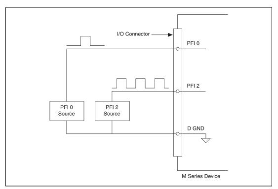
Figure 8-3. PFI Input Signals Connections
